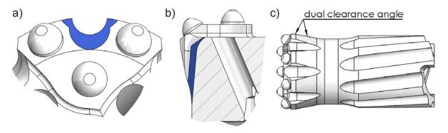
Simulation analysis identified flushing as a key performance factor for the medium to large end button bits. Picture highlights these development aspects of the Evolution bit, where (a) the side flushing grooves are deeper and give space for a smoother transition region, and (b) the overall side channel volume is increased. In addition, the (c) dual clearance angles were tweaked for even more flow over the sides and extra support for the buttons.
