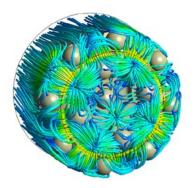
Computational Fluid Dynamics (CFD) simulation images showing how the conventional model (left) has a dead space in the center of the bit where airflow velocities are low. Evolution model (right), with a more even flow pattern, has increased airflow at the center of the bit and through the secondary side channels.
